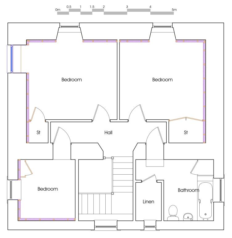
Proposed First Floor Layout Plan Scale 1:50
