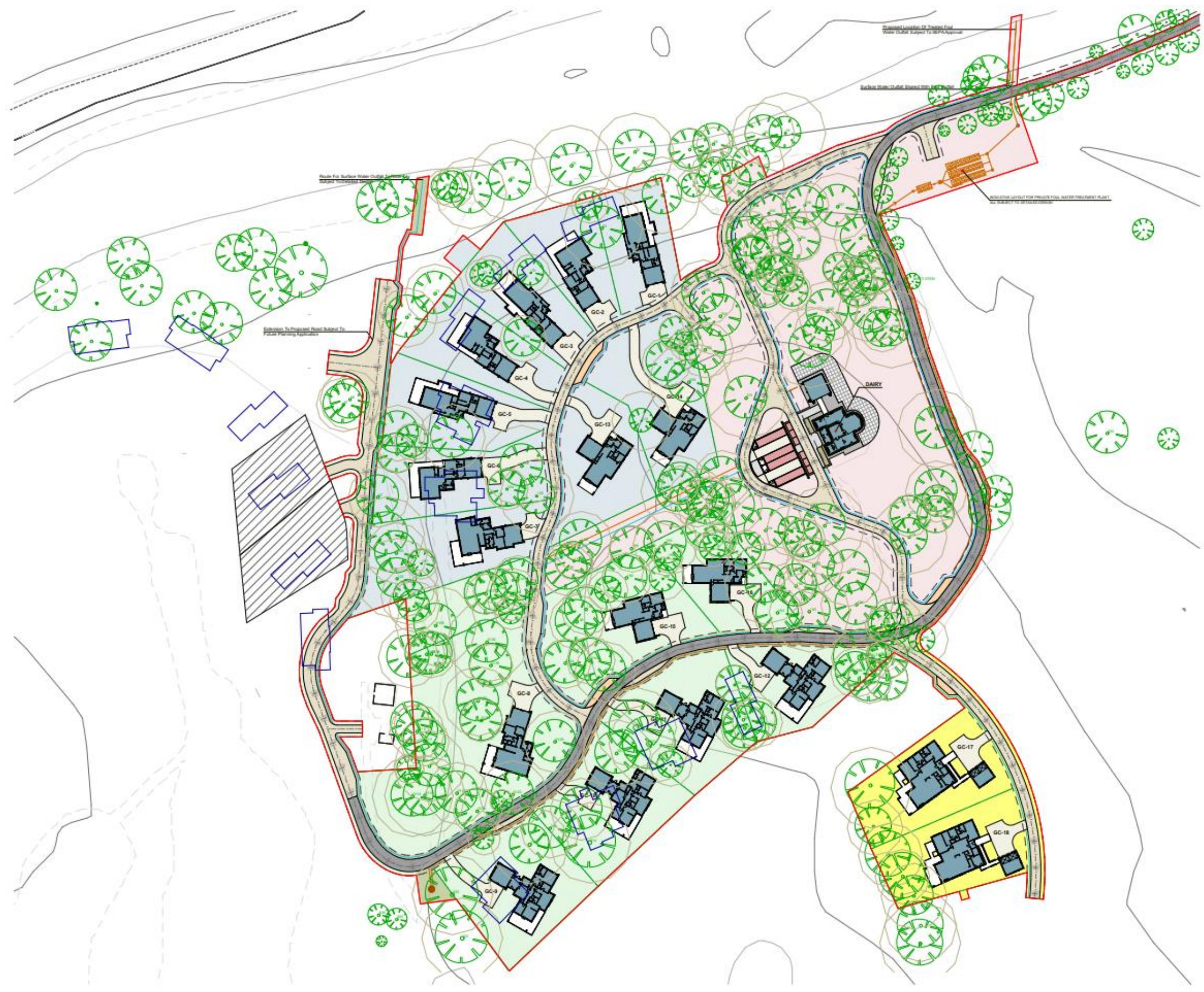
Extract from Site Masterplan drawing showing proposed house footprints in blue fill, with previously consented house footprints illustrated in blue outline for comparison.
