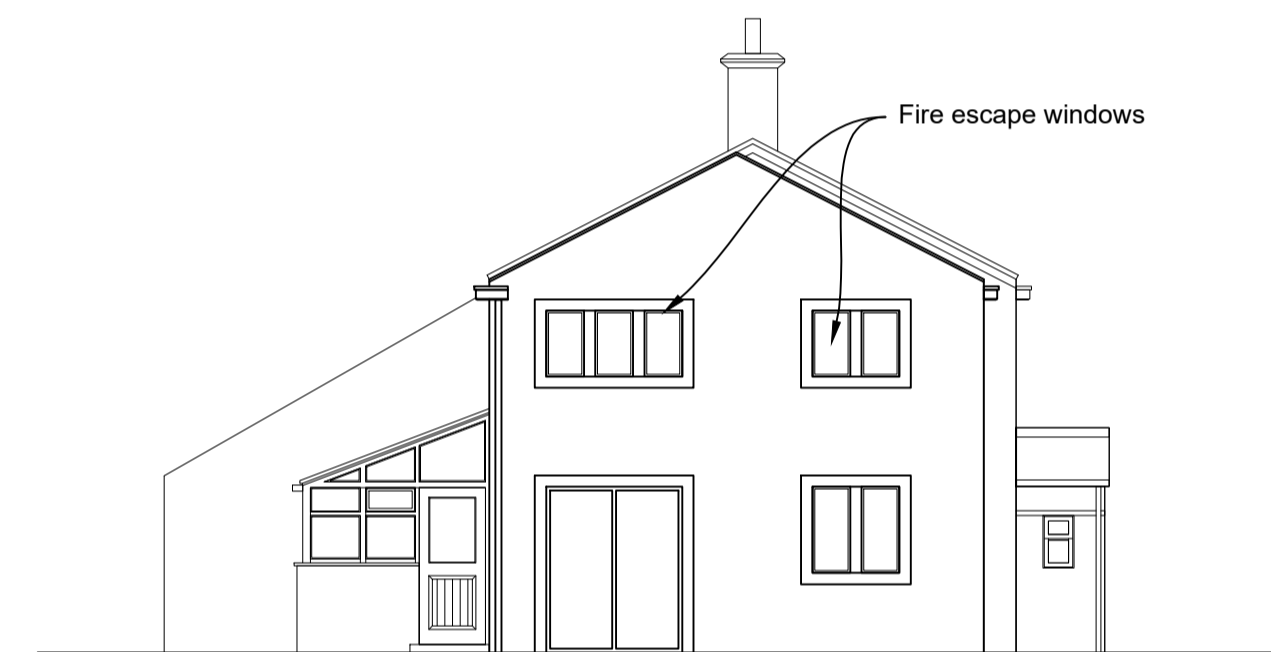
South West Elevation
