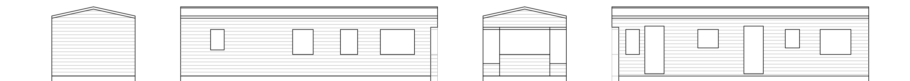
Welfare Unit Side Elevation As Existing/Proposed Welfare Unit Front Elevation As Existing/Proposed Welfare Unit Side Elevation As Existing/Proposed Welfare Unit Rear Elevation As Existing/Proposed
