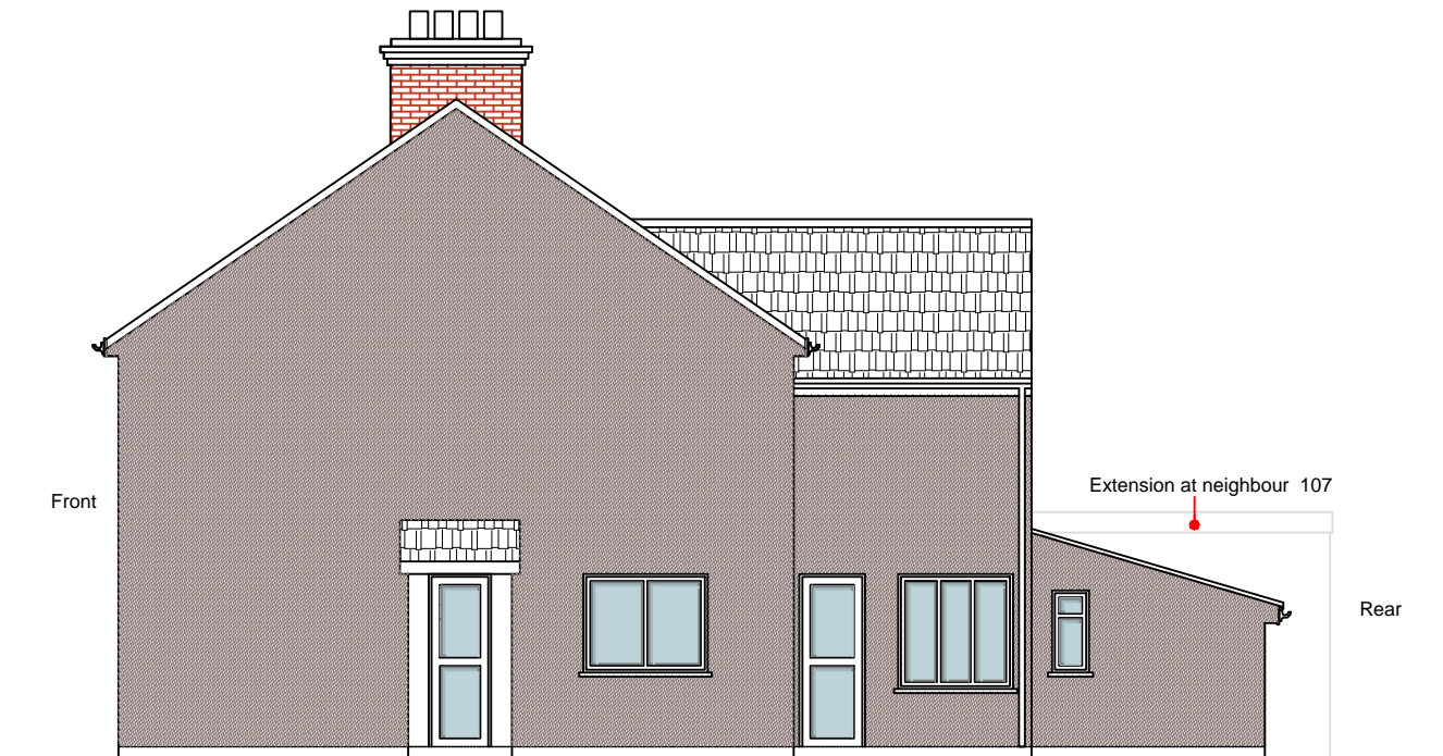
EXISTING SIDE ELEVATION
