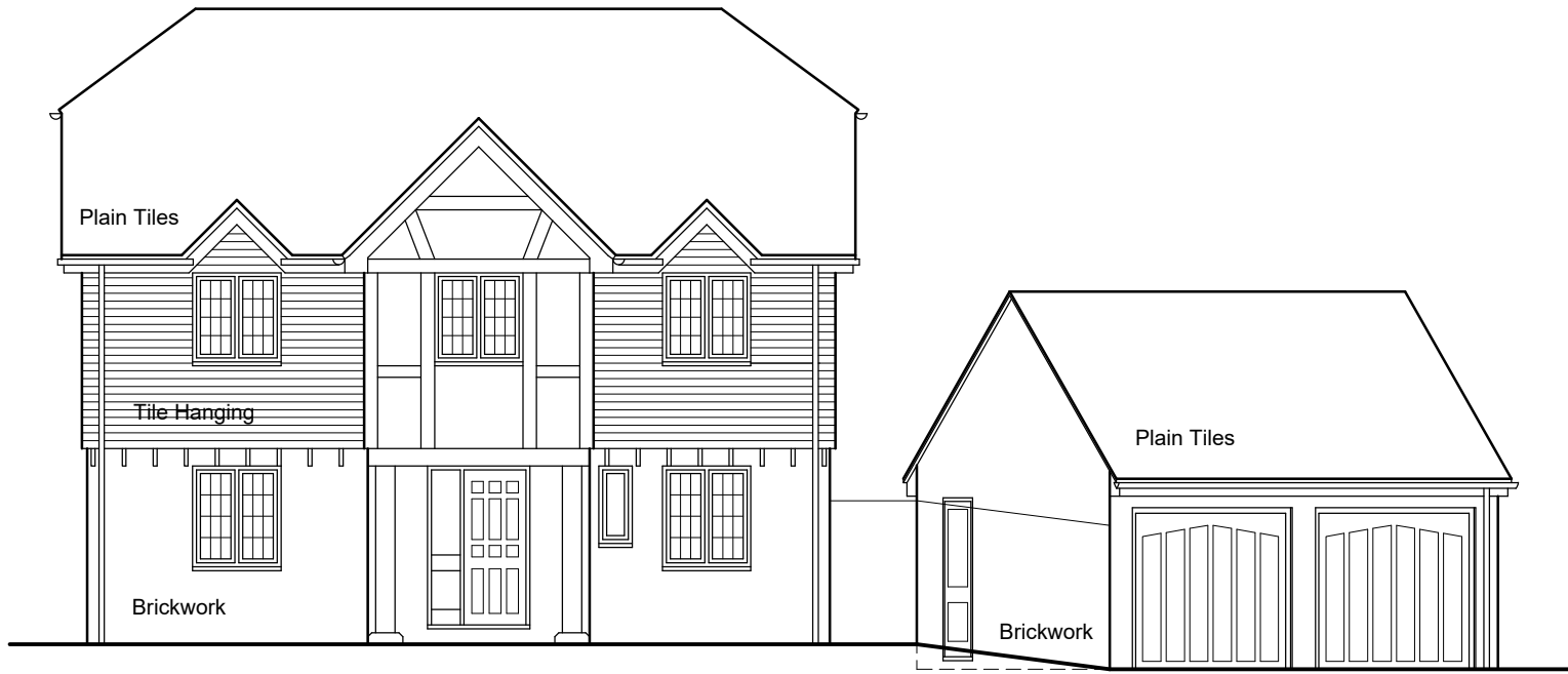
Front Elevation Existing
