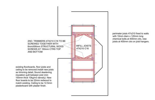
FIRST FLOOR TRIMMING DETAIL denotes metal joist hangers / angle brackets fully fixed
