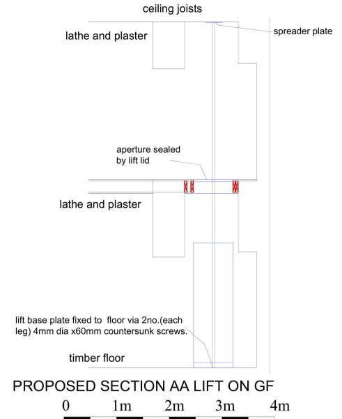
Guide top spacer (lift legs) fixed to ceiling
