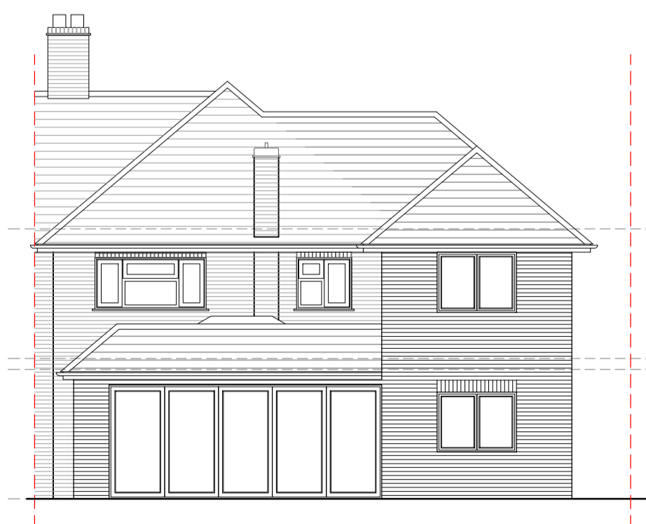
Rear Elevation SCALE 1:100
