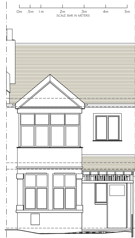
EXISTING FRONT ELEVATION
