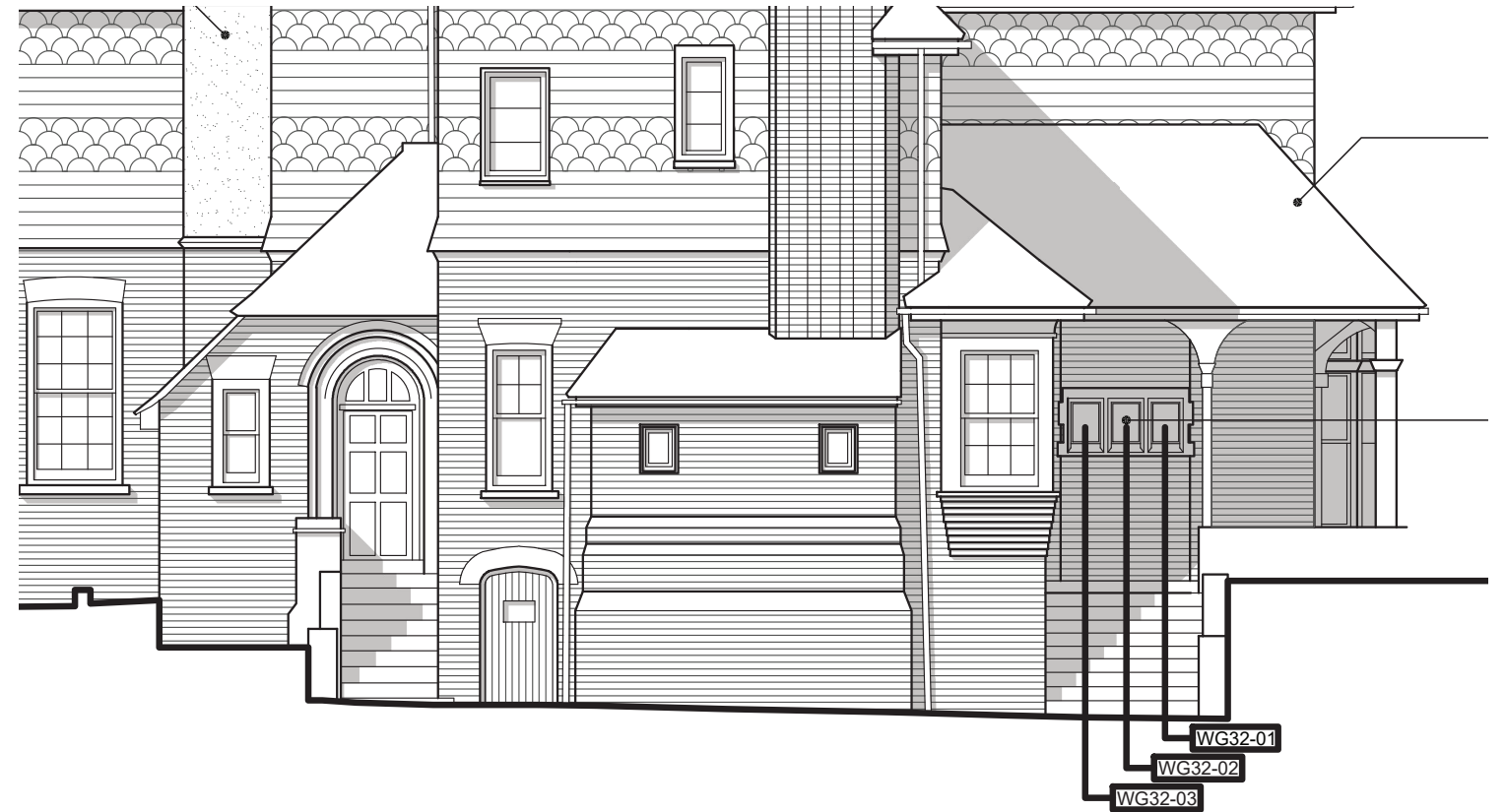
Part proposed West elevation showing the proposed relocation of window WG32
