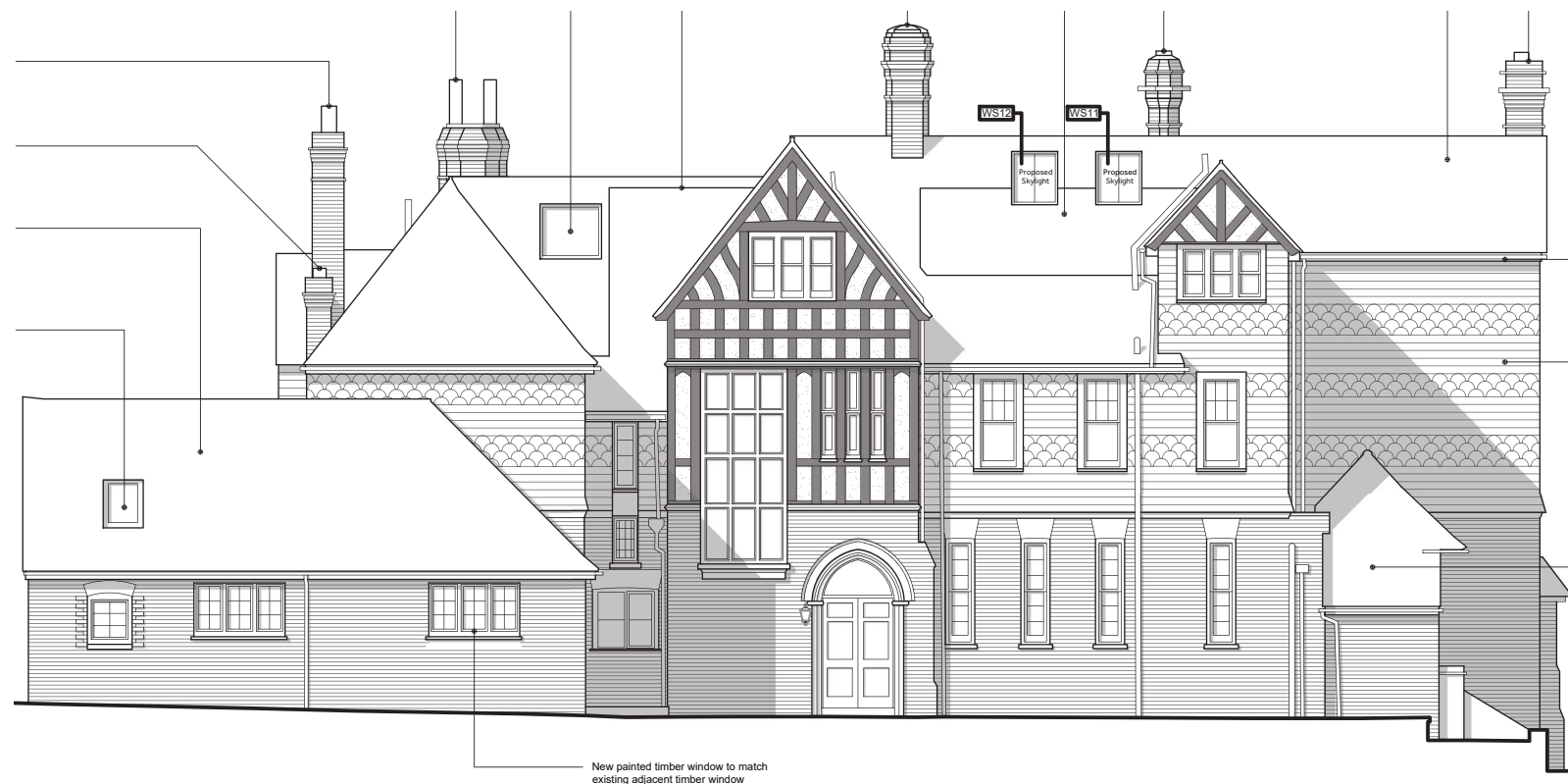
Proposed North Elevation with the dormer window and lightweight roof access enclosure removed.
