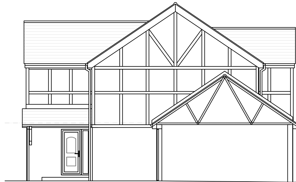
EXISTING SECTION D - THRU' GARAGE
