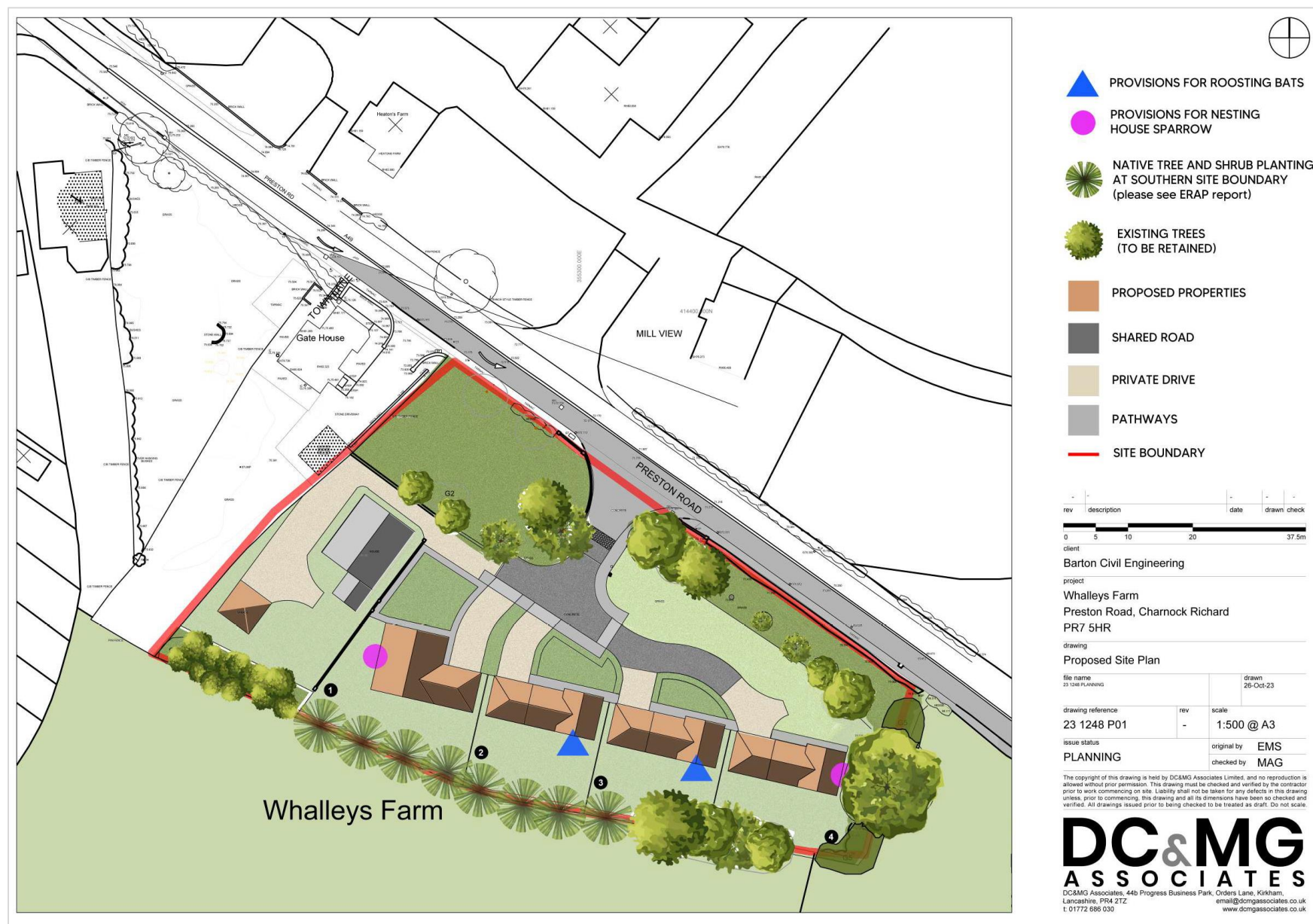
Figure 3: Proposed Site Plan with Suggested Locations of Bird Boxes and Bat Access Panels
