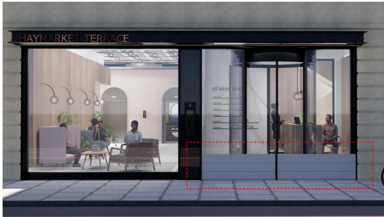
Elevation 1: Flood Barrier – Manually Installed (consented)
