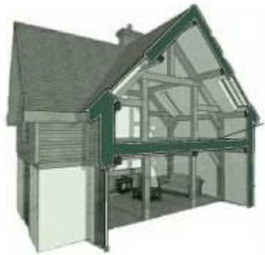
Highly Insulated Airtight Thermal Shell
