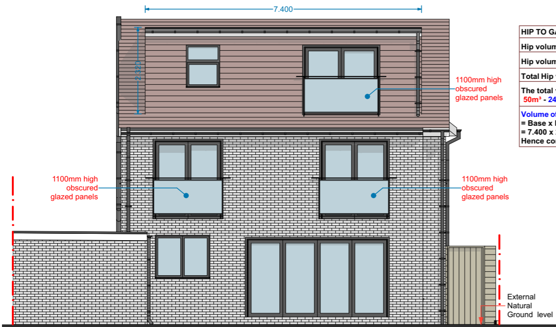
Existing (As Built) Rear Elevation 1:100
