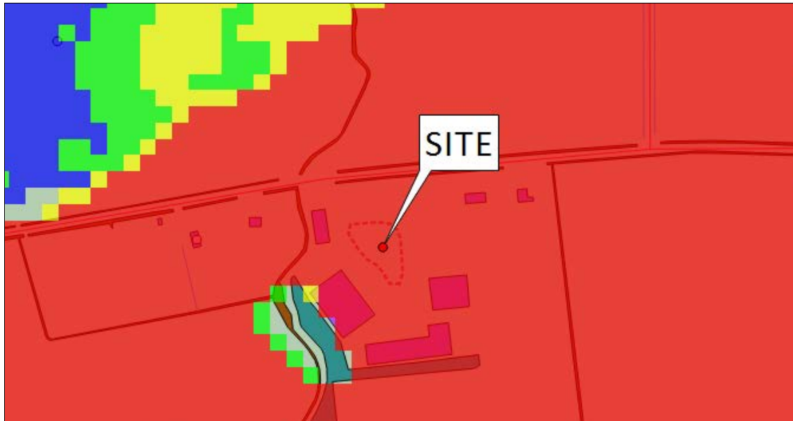
Defended Overtopping Hazard 0.5% AEP With Climate Change – Red Indicates High Hazard
