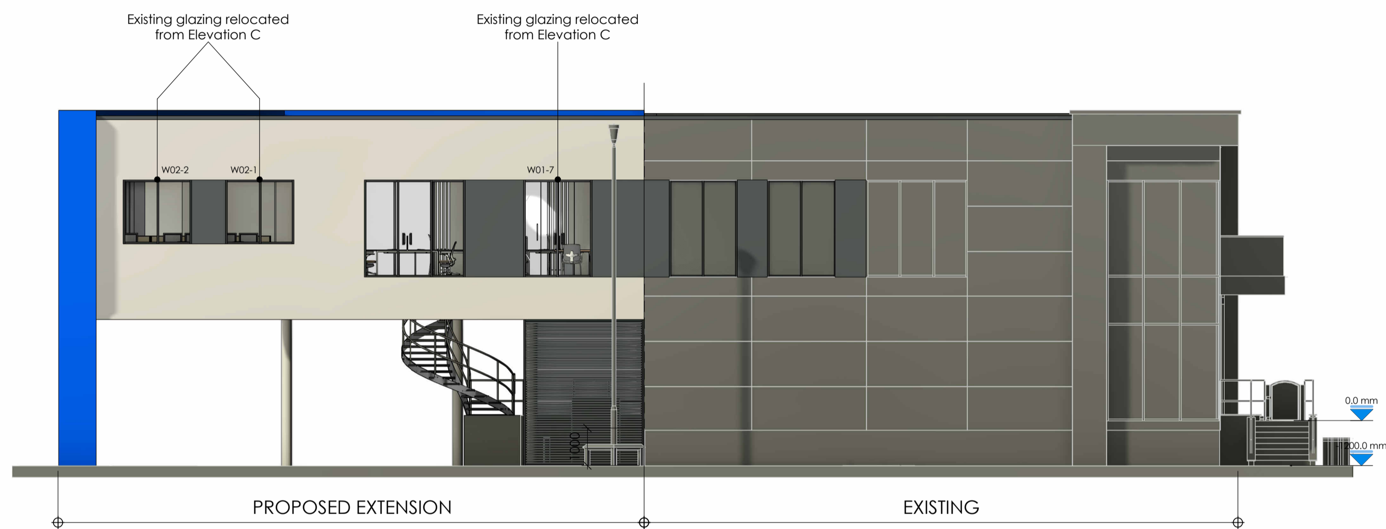
B Elevation B - Proposed Extension Work 1 : 100
