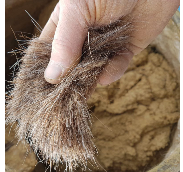
Goat/horse hair can be added to lime plasters and renders to give extra tensile strength
