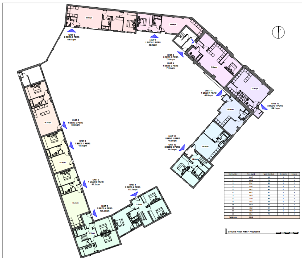
Figure 2.2 – Proposed ground floor plan.
