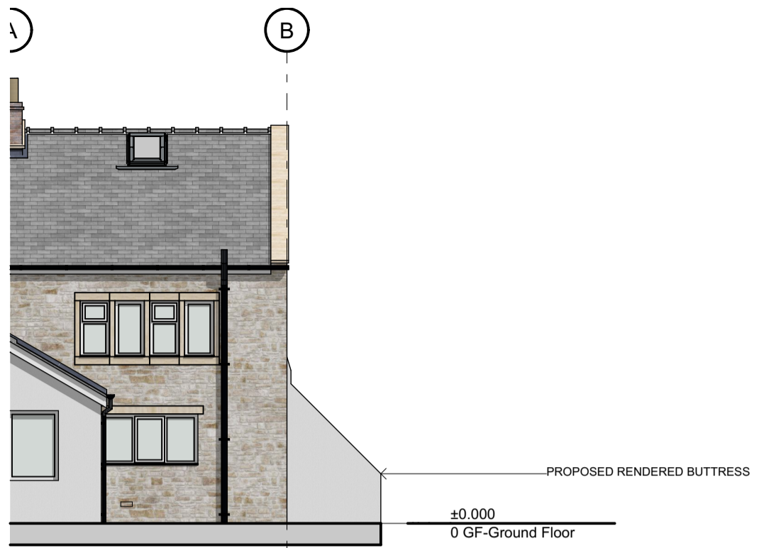
NORTH EAST Elevation 1:100
