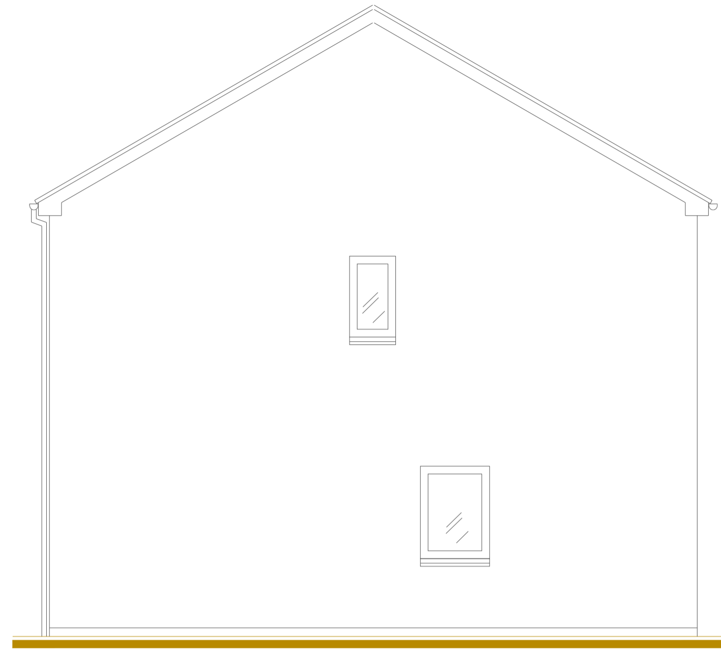
EXISTING NORTH FACING ELEVATION (scale 1:50)
