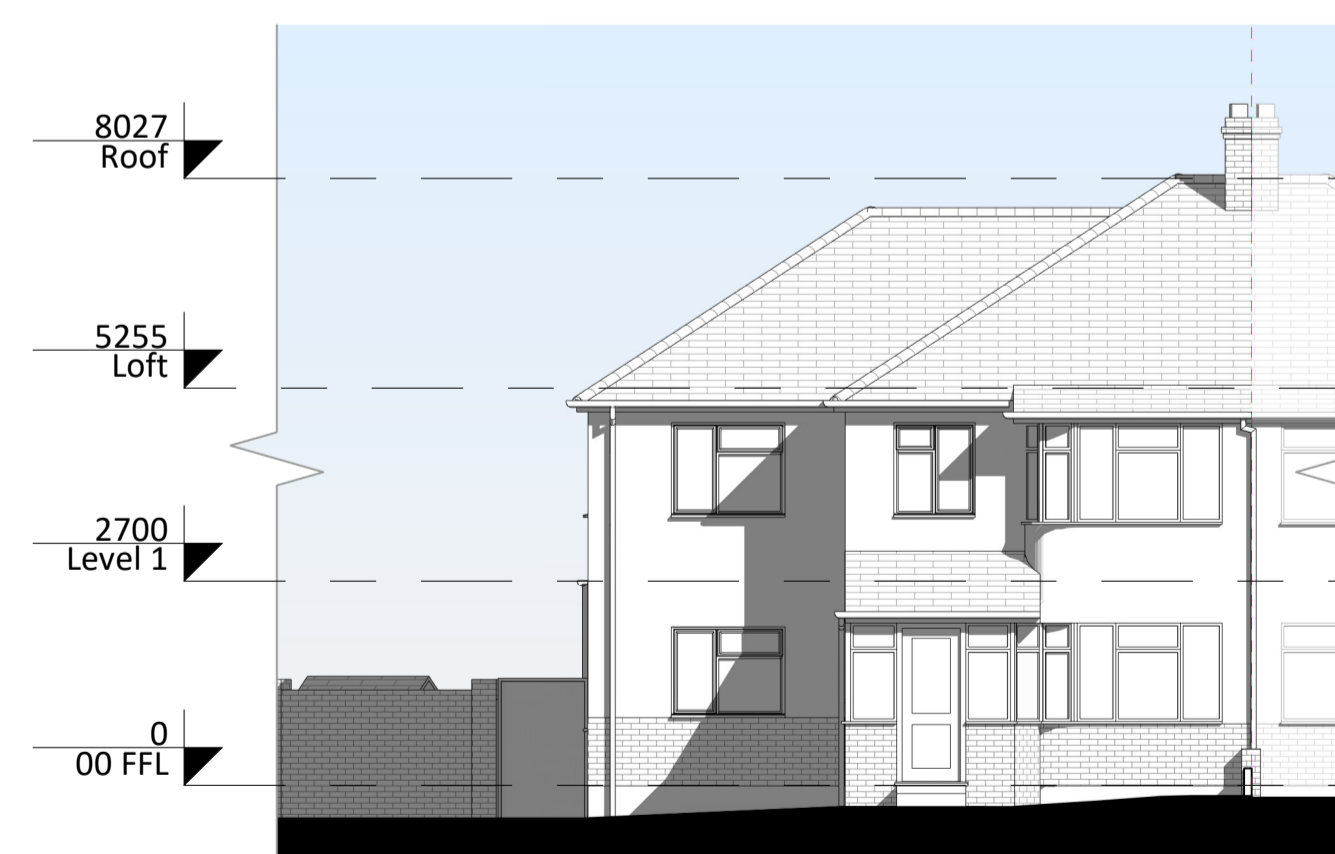
5 Existing Front Elevation 1 : 100
