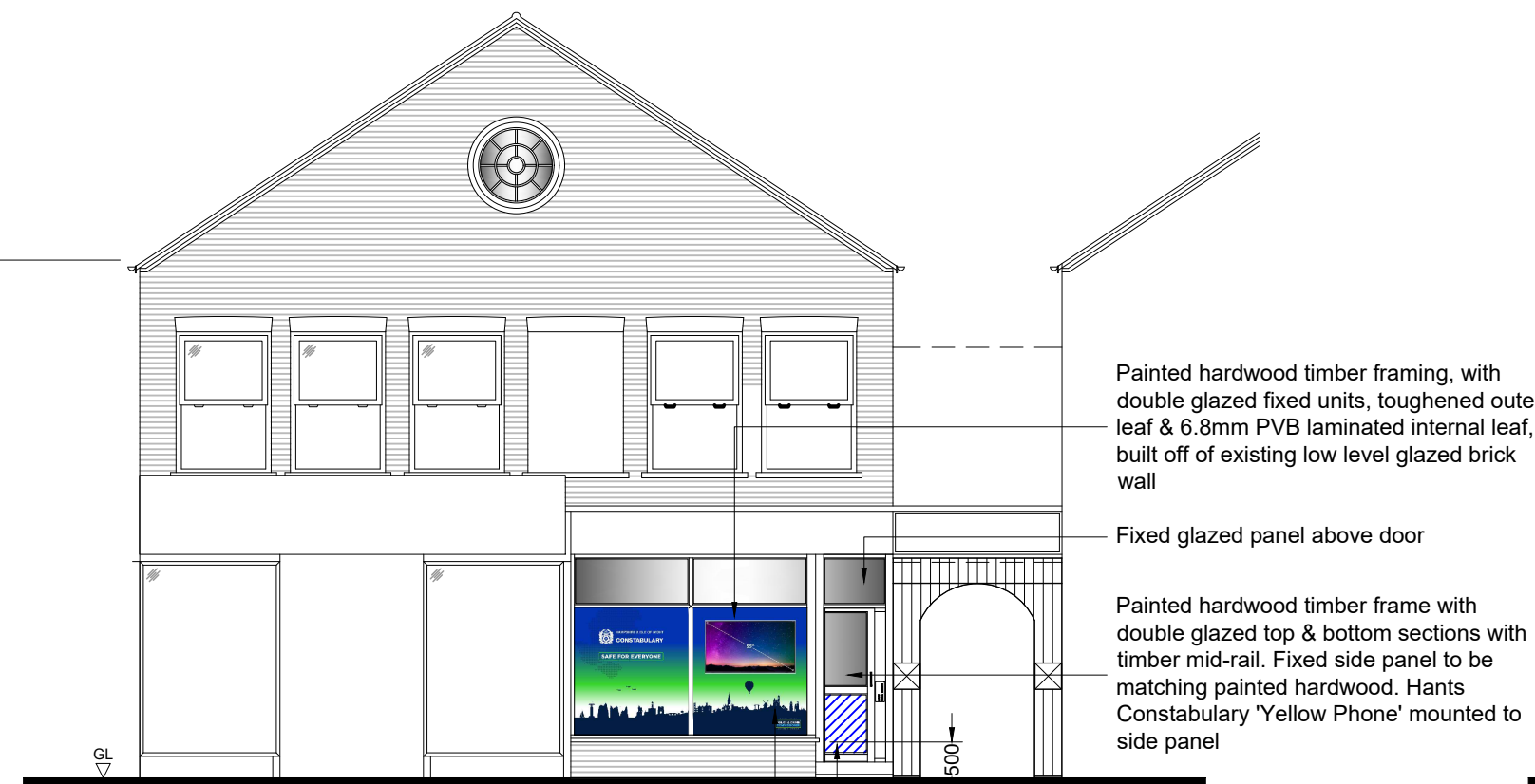
EXISTING FRONT (WEST) ELEVATION (1:100)
