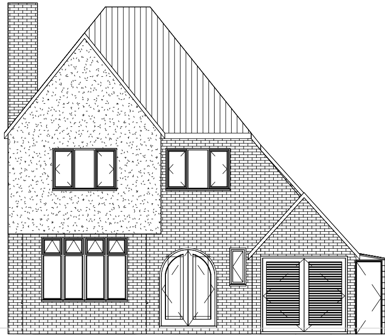
1 Existing Front Elevation 1 : 100
