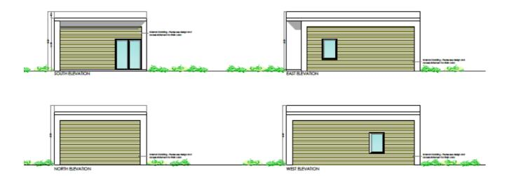
The studio will be installed on concrete foundations and built from lightweight steel and clad in weatherboarding. The roof will be rubber membrane with Photo Voltaic panels surface mounted.
