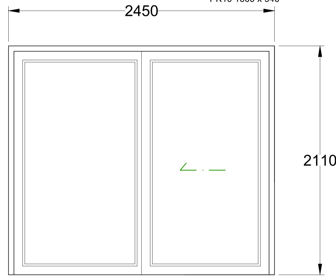
Double glazed timber sliding patio doors Velfac 200 or equal and approved 1:20 RAL 7034 yellow-grey
