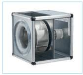
In the GigaBox T120 range, the motor is located outside the delivery flow and is separated from the impeller by a heat-insulated wall. The motor impeller unit can be removed without dismantling the ducting system.
