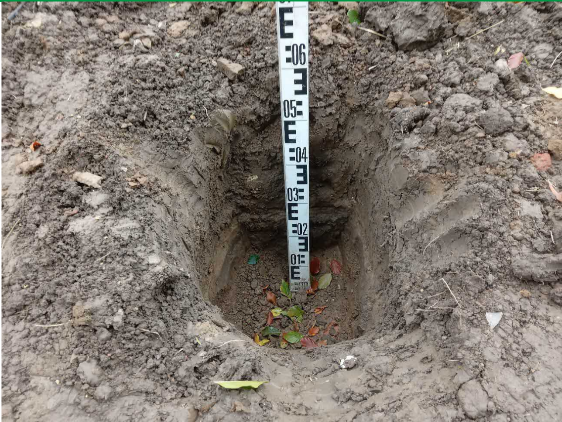
PLATE 5 – PLACED TOPSOIL MATERIALS AND DEPTH VALIDATION OF PLOT 11
