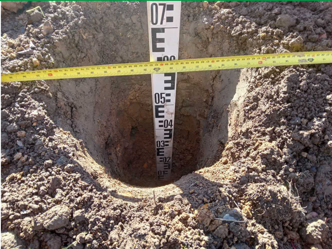
PLATE 1 – PLACED TOPSOIL MATERIALS AND DEPTH VALIDATION OF PLOT 1
