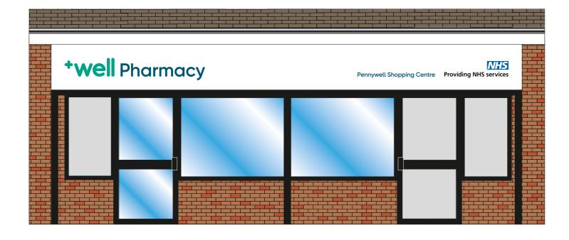
4No. Non-Illuminated folded dibond tray panel @ 6994 x 680mm including 20mm upstand with 25mm returns, complete with 5mm Acrylic cut our Well logo & Pharmacy text on stand off locators.
