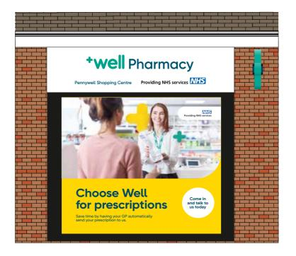
4No. Non-Illuminated folded dibond tray panel @ 2800 x 680mm including 20mm upstand with 25mm returns, complete with 5mm Acrylic cut our Well logo & Pharmacy text on stand off locators.
