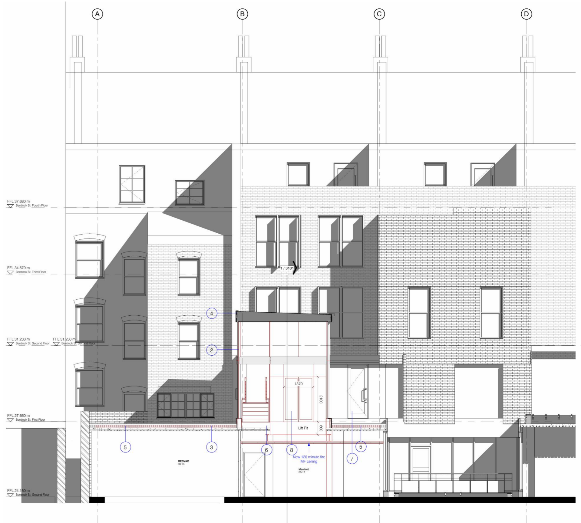
Proposed Elevation showing the extent of the proposal as a 2700mm above the Wigmore Street second floor.
