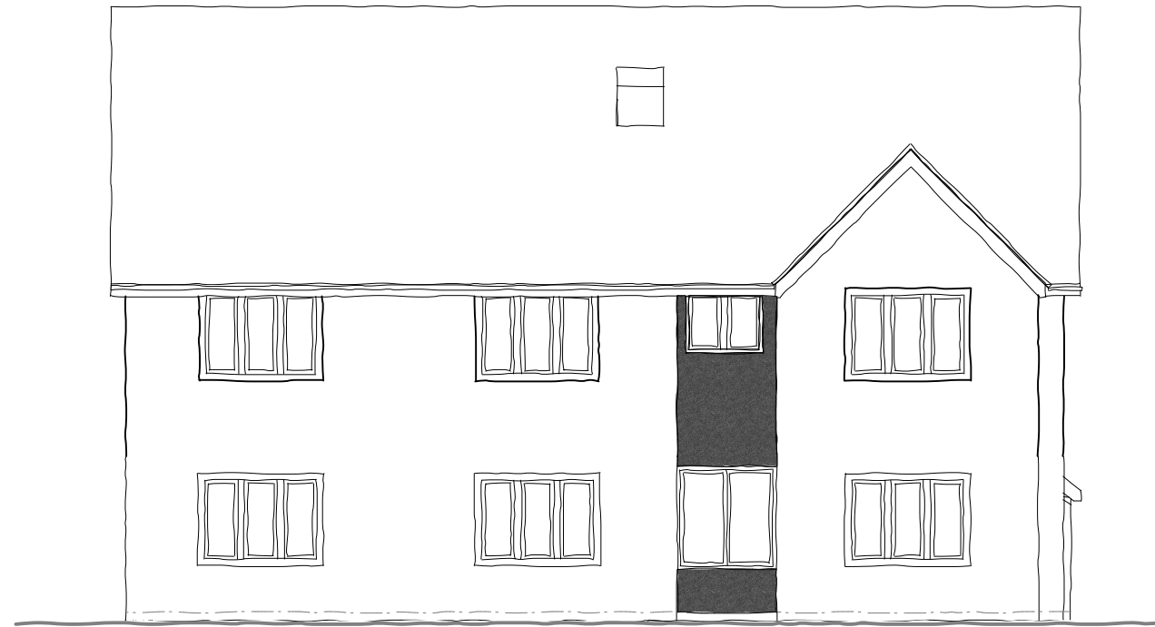
remove canopy clad recess
