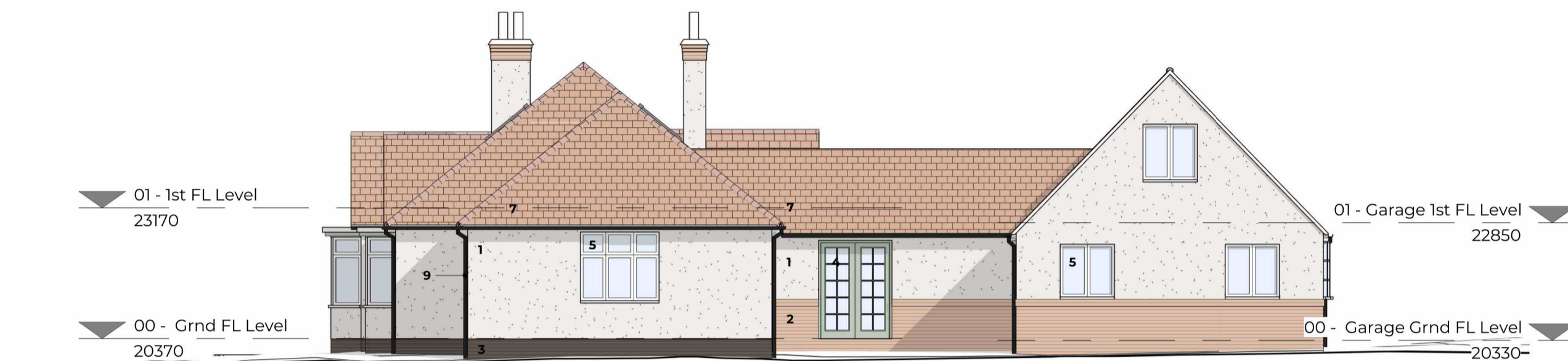
Proposed East Elevation 1:100
