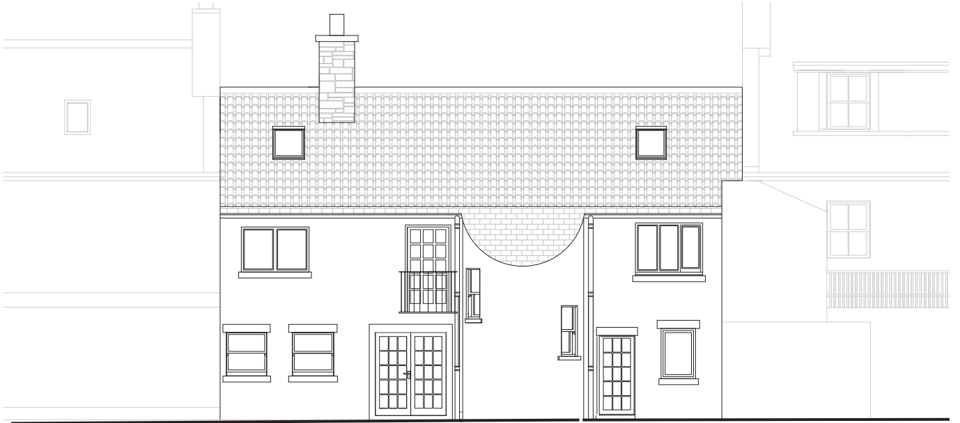
60. Existing Rear Elevation Presenting a wide variety of openings in styles, proportions and detailing. The proportions and styles are at odd with the character and date of construction of the house. There is no consideration for traditional elevation lay-out and geometry
