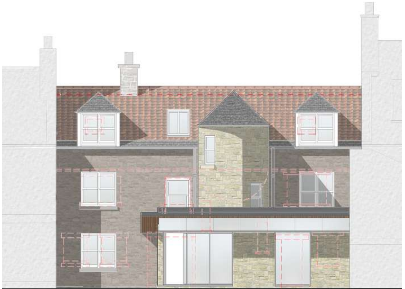
62. Revised Design - The proposal is to harmonise the existing elevation and staircase extension to create a historical ensemble with traditionally proportioned and detailed windows, dormers and vertical elements. This allows for a more engaging contrast with the proposed ground floor extension.
