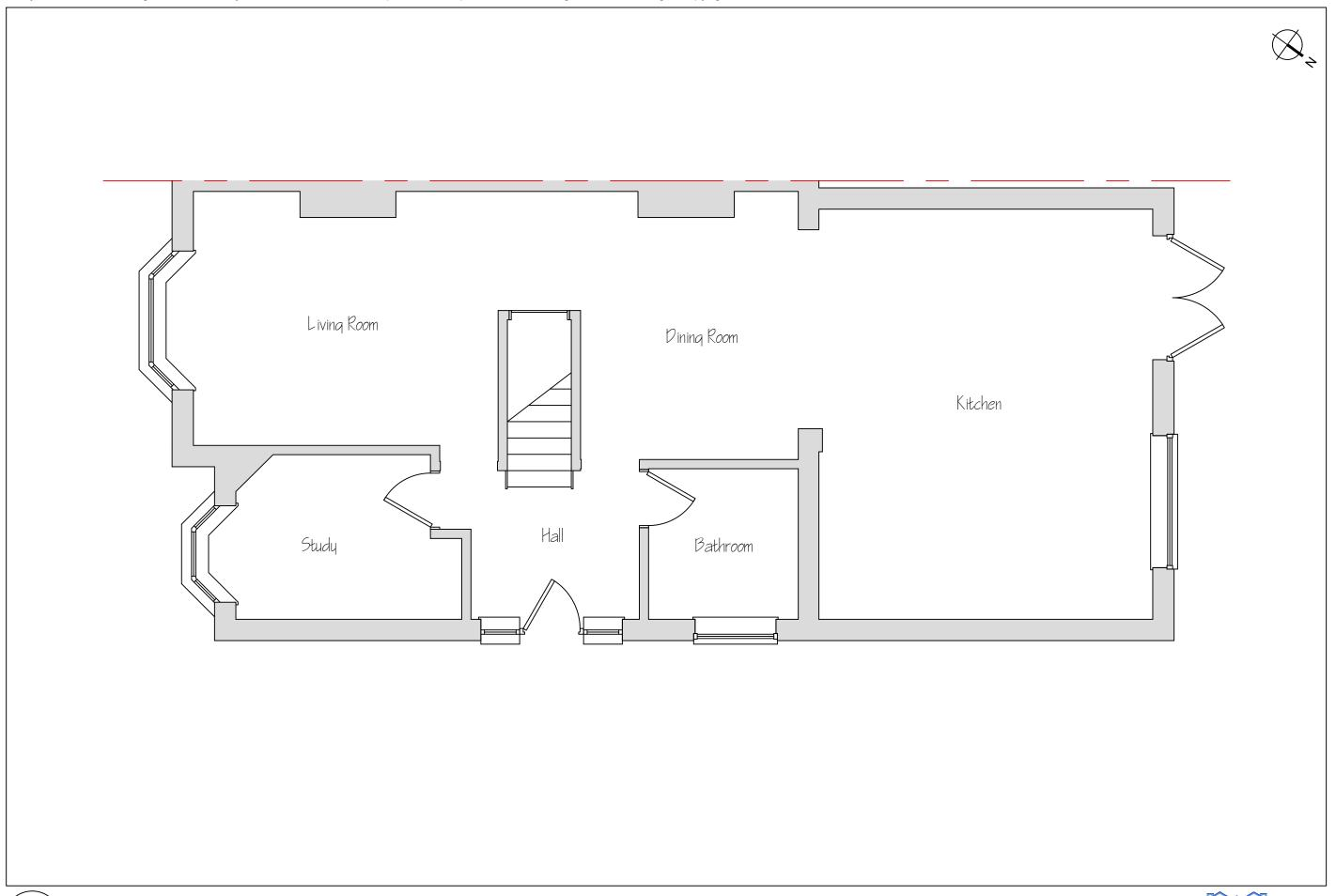
Existing & Proposed Plans: Ground Floor (E-(01)00 (Scale 1:50 @A3) Meters
