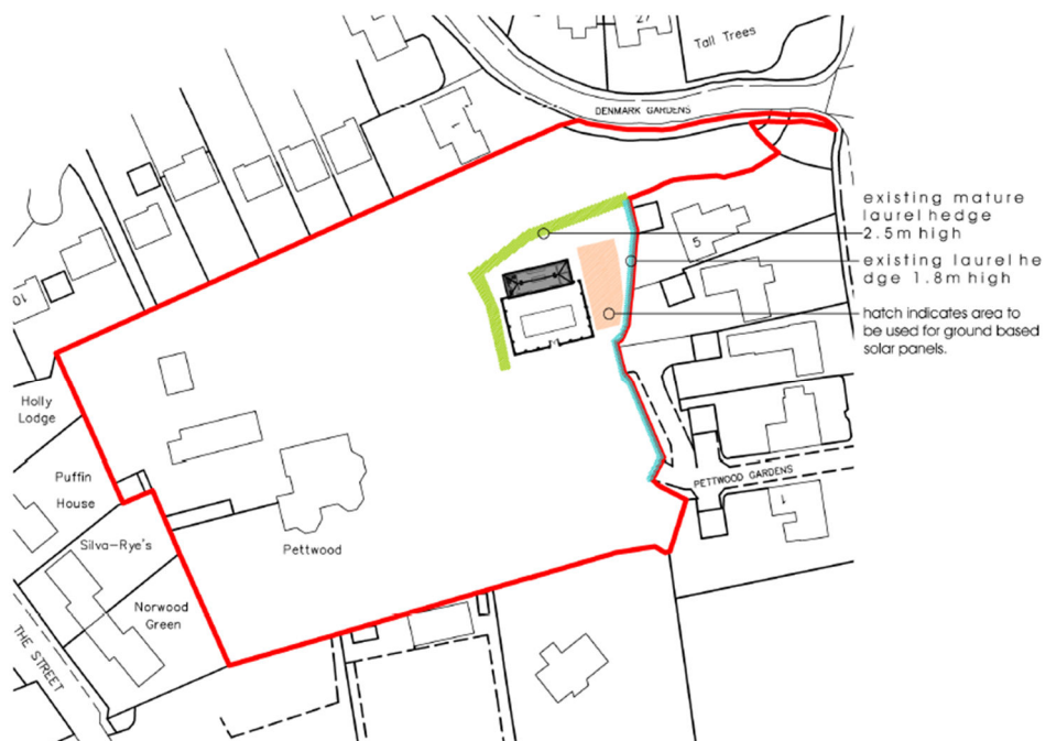
Block plan showing proposed area (orange hatch) is screened from three sides.
