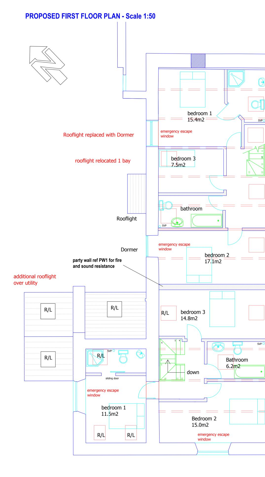
Scale 1:50 (metres) Rooflight Rooflight 2no rooflights relocated Rooflight R/L Unit 4 GF only Rooflight Light Jube R/L light tube to bathroom Rooflight 1no rooflight relocated 8246 SVP 🔿 Airing Cup'd ° T R/L office/study 6.5m2 R/L R/L Ensuite Master Suite 20.1m2 🖾 down down  $\rightarrow$ \_\_\_\_ • °°° Bedroom 3 7.5m2 Bedroom 2 Bathroom 11.5m2 6.6m2 R/L R/L R/L SVP Rooflight replaced Rooflights Rooflight replaced with Dormer with Dormer
