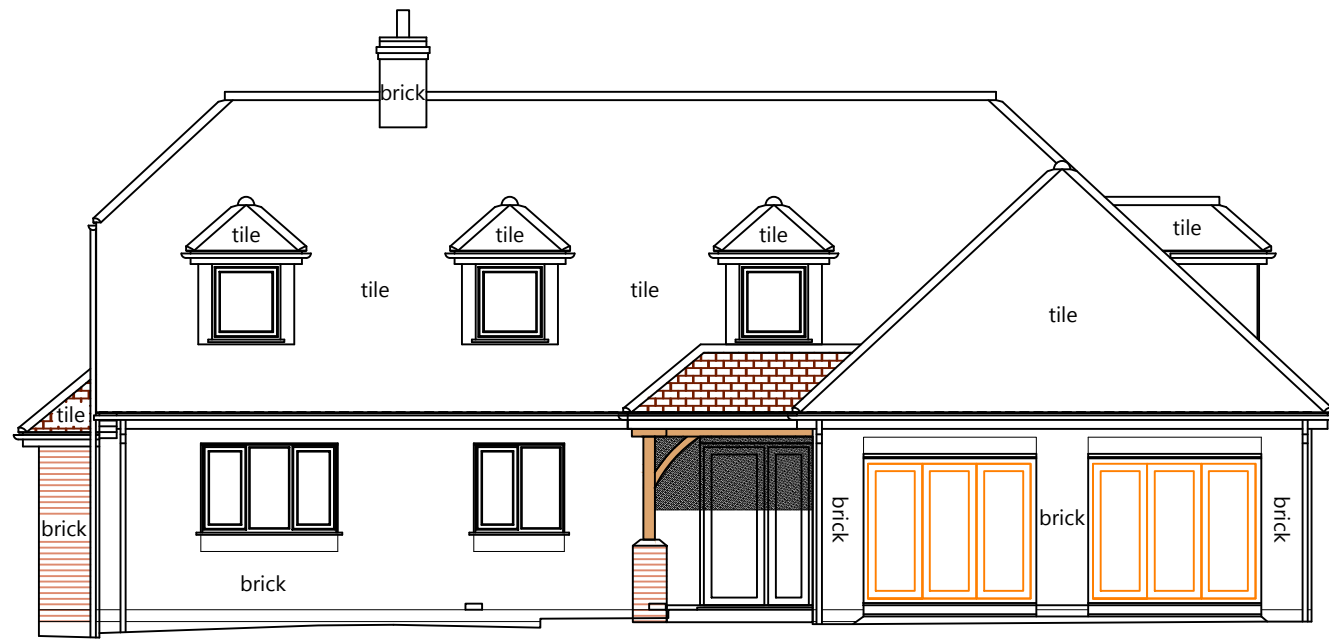
Elevation 1 SOUTH EAST ELEVATION
