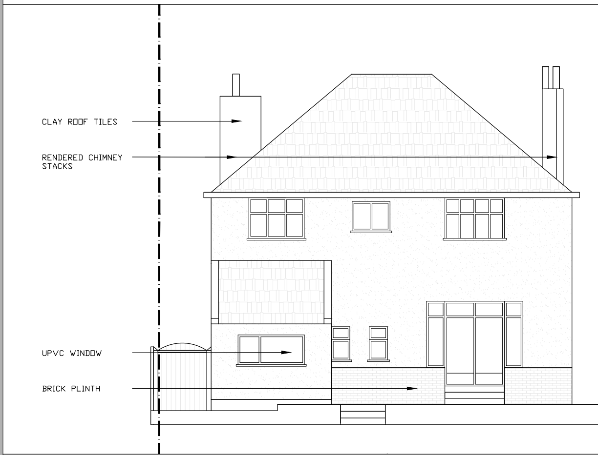
SOUTH EAST ELEVATION - EXISTING
