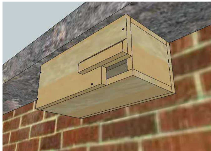
Figure 12: Swift box, source: http://actionforswifts.blogspot.com/p/diy-swift-box-designs.html
