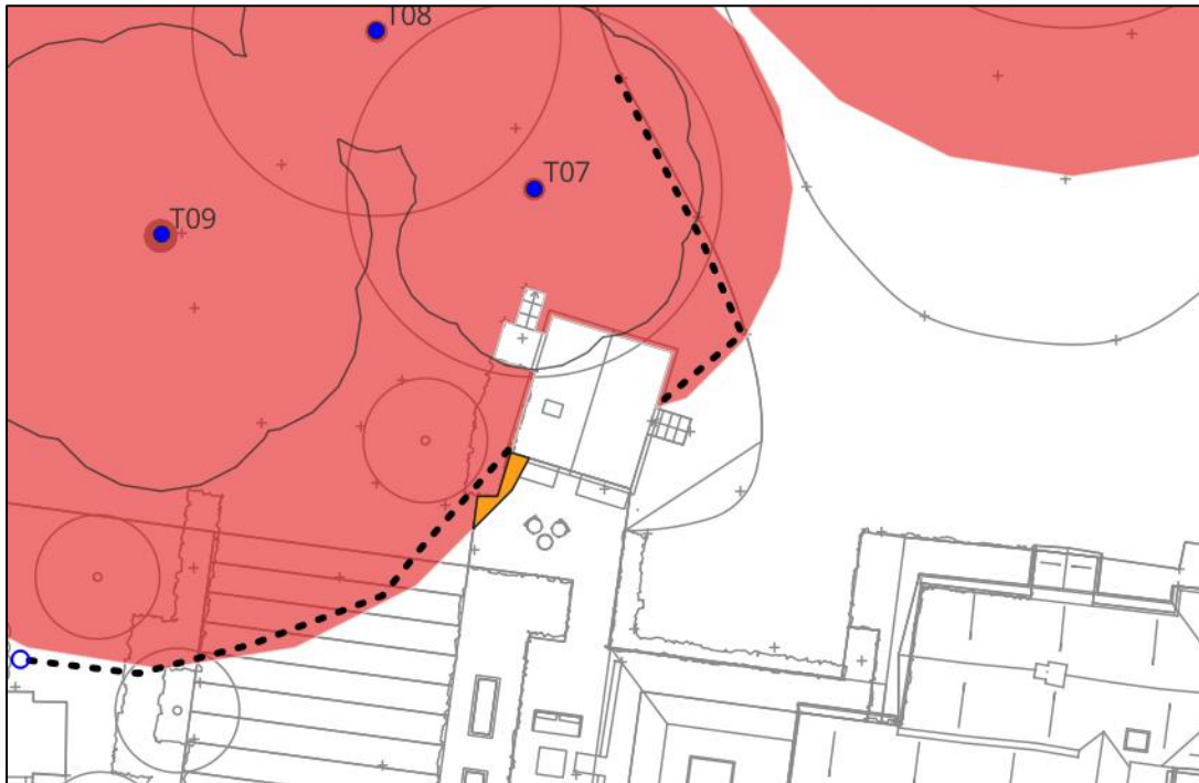
Fig 2: Recommended temporary barrier (dashed line) to prevent construction encroachment within root protection areas of adjacent trees.
