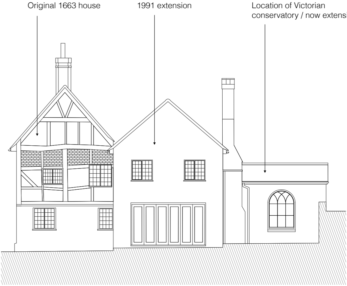
Existing western elevation, not to scale
