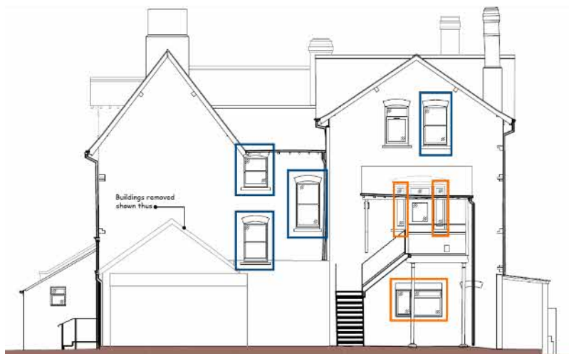
Plate 15: Southeast elevation with the location of sash windows outlined in blue and single glazed window units of no heritage interest outlined in orange.
