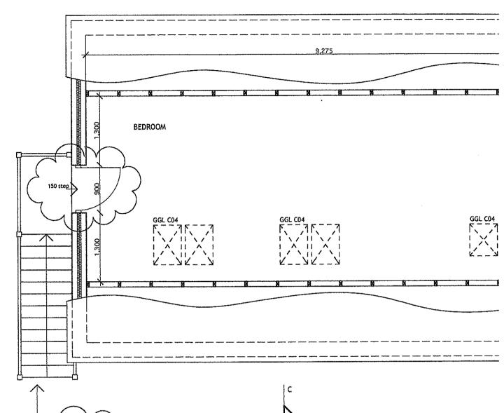
Timber framed staticase with 1800mm high vertical 'hit & miss' timber fence screening to sides and end to retian privacy of immediate neighbours
