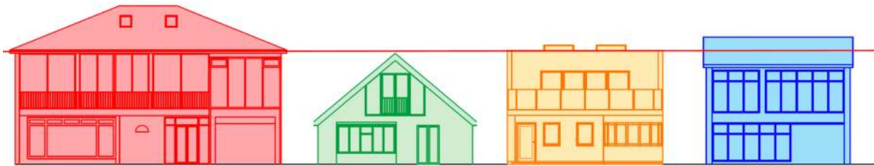
Annotated extract of drawing 2820-08-1 [not to scale] - red line marks the ridge height of the proposed building and demonstrates its congruent relationship with neighbours
