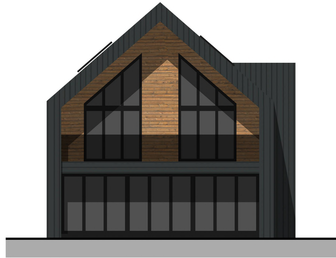
proposed side elevation 2 dwelling 1 scale 1:100
