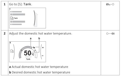
When weather-dependent operation is used for the tank, the tank temperature is determined automatically by the outdoor temperature. For more information, see "5.9 Weather-dependent curve" [> 46].
