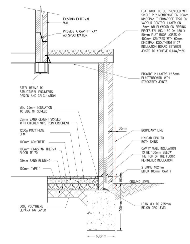
PROPOSED SECTION A-A THROUGH SINGLE STOREY REAR EXTENSION SCALE 1:20
