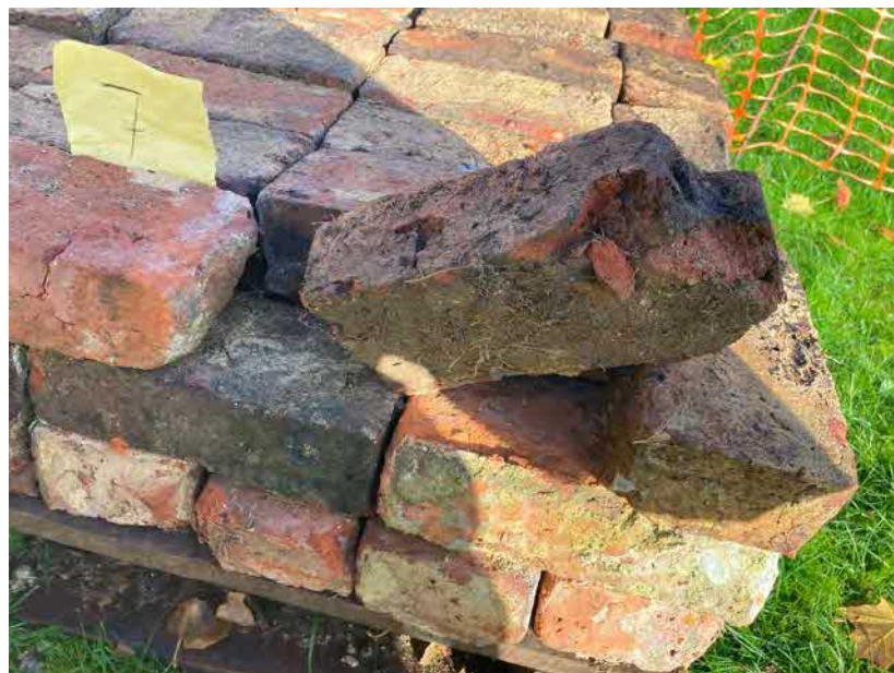
Stack 7 selected for reuse subject to final selection during laying* *have at least one good face on the stretchers on original inspection but could expect some limited rejections during the laying process
