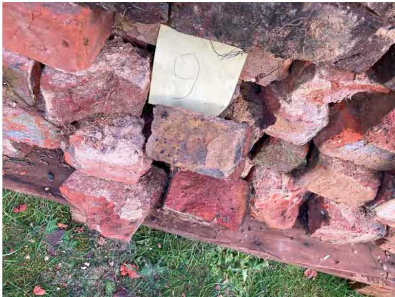
Stack 9 - rejected subject to final hand sort during disposal in case Any better bricks are in the centre of the stack
