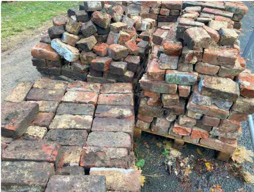
Stack 4 - rejected subject to final hand sort during disposal in case any better bricks are in the centre of the stack
