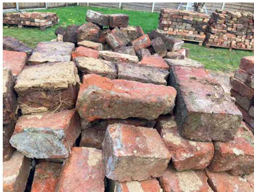
Stack 5 - rejected subject to final hand sort during disposal in case any better bricks are in the centre of the stack
