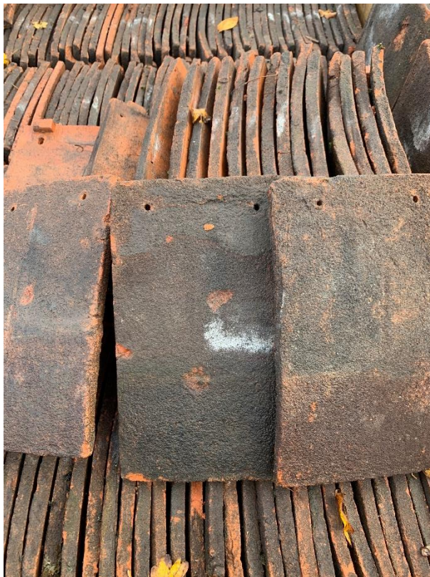
Fig 14. ROOF: Reclaimed clay tiles
